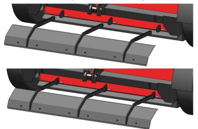
3/8" x 1.75" - Grader link 1 - 3/8" washer - Mounting tab - 3/8" washer - Grader link 2 - 3/8" nut
